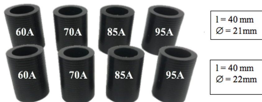
Fig. 3.20 The set of idealised compliant phantoms 3D printed with PolyJet technology.
