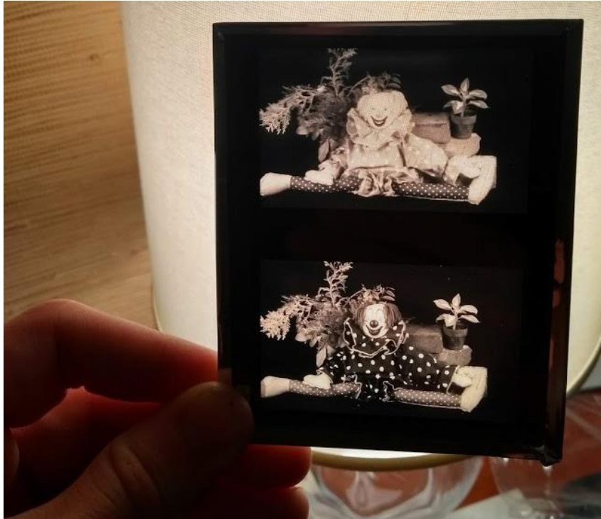
Figure 3: Two pictures, the top taken through a red filter, and the bottom taken through a green filter. Image: Taken by the author during a visit to John McCann (former head of the Polaroid Vision Research Laboratory) in July 2018. Permission from John J. McCann.
