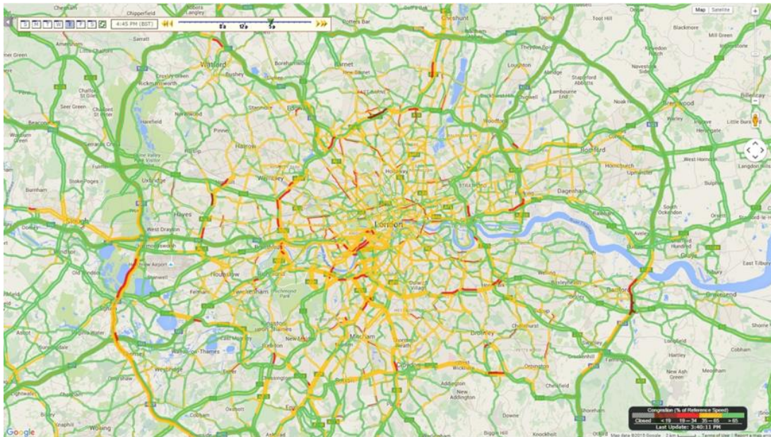
Figure 1. INRIX Congestion Index for Peak Period Travel in London [dark red = worst]
