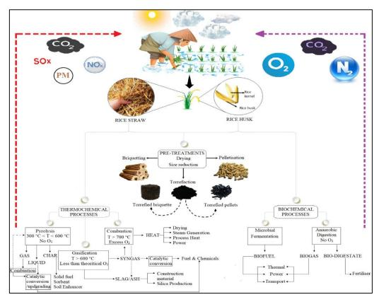
**Figure 1.** Rice husk and rice straw conversion through thermochemical and biochemical processes. Note: SOX (sulphur oxides), PM (particulate matter), NOX (nitrogen oxides), CO<sub>2</sub> (carbon diox-ide), O<sub>2</sub> (oxygen), N<sub>2</sub> (nitrogen).
