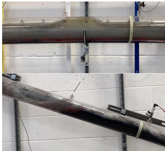
Figure 4.12 Difference in solid particle transport mechanisms for the same air-water flowrate ( Q_m=38\text{m}^3/\text{hr} , C_c=4\text{-}10\% by volume, \text{RPM}=0 , e=0 ) for slug flow pattern with a moving bed, in a horizontal annulus ( \theta=0^\circ ) (top), and stationary bed in an inclined annulus ( \theta=30^\circ ) (bottom)
