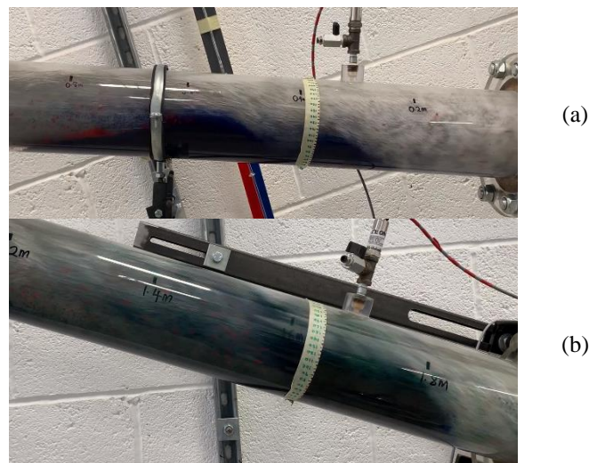
Figure 4.8 Dispersed bubble flow pattern at the same air-liquid flowrate ( Q_m=42\text{m}^3/\text{hr} , C_c=4\text{-}10\% by volume, \text{RPM}=0 , e=0 , \theta=30^\circ ) (a) air-water mixture with a moving bed solid particle mechanism, and (b) air-polymer mixture with suspension solid particle mechanism
