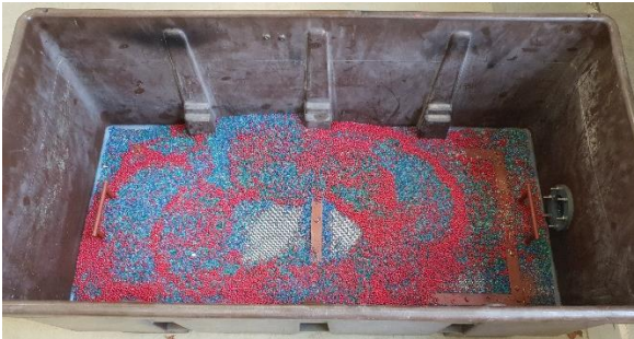
Figure 3.11 Photo of solids separation tank with the solid particles which have different sizes and densities
