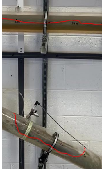
Figure 4.10 Difference in gas-liquid flow pattern distribution at same air-water flowrate ( Q_m=40\text{m}^3/\text{hr} , C_c=0\% by volume, \text{RPM}=0 , e=0 ), stratified flow in a horizontal annulus ( \theta=0^\circ ) (top), and slug flow in an inclined annulus ( \theta=30^\circ ) (bottom)
