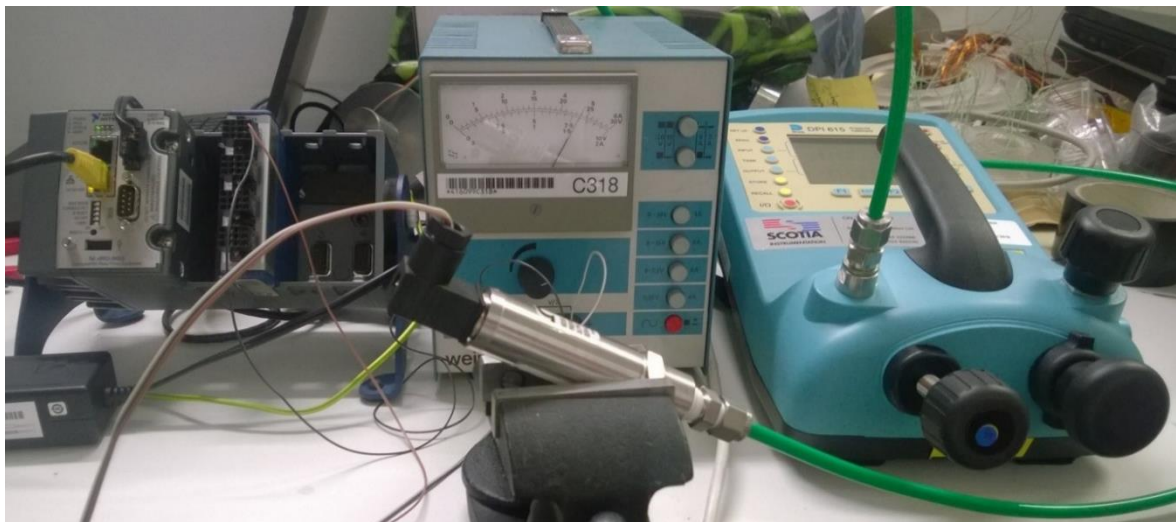
Figure. A.1 Pressure transducer calibration setup
