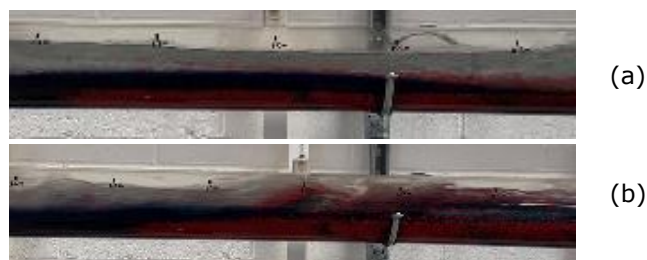
Figure 4.7 Flow pattern with different gas-liquid input flowrates (a) stratified flow ( Q_m=35\text{m}^3/\text{hr} , C_c=4\text{-}10\% by volume, \text{RPM}=0 , e=0 , \theta=0^\circ ), and (b) slug flow ( Q_m=42\text{m}^3/\text{hr} , C_c=4\text{-}10\% by volume, \text{RPM}=0 , e=0 , \theta=0^\circ )
