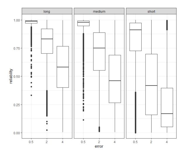
Figure 5.3: Distribution of reliability values pooled across all metrics from in silico experiments created with error magnitudes of 0.5, 2 and 4 metres and attack time grouping (short: <10 s, medium: 10-20 s, long: >20 s).
