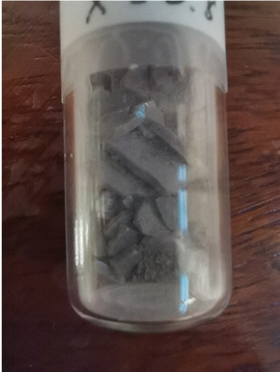
Figure 8-1: NTSP glass with composition x = 1.0 .
