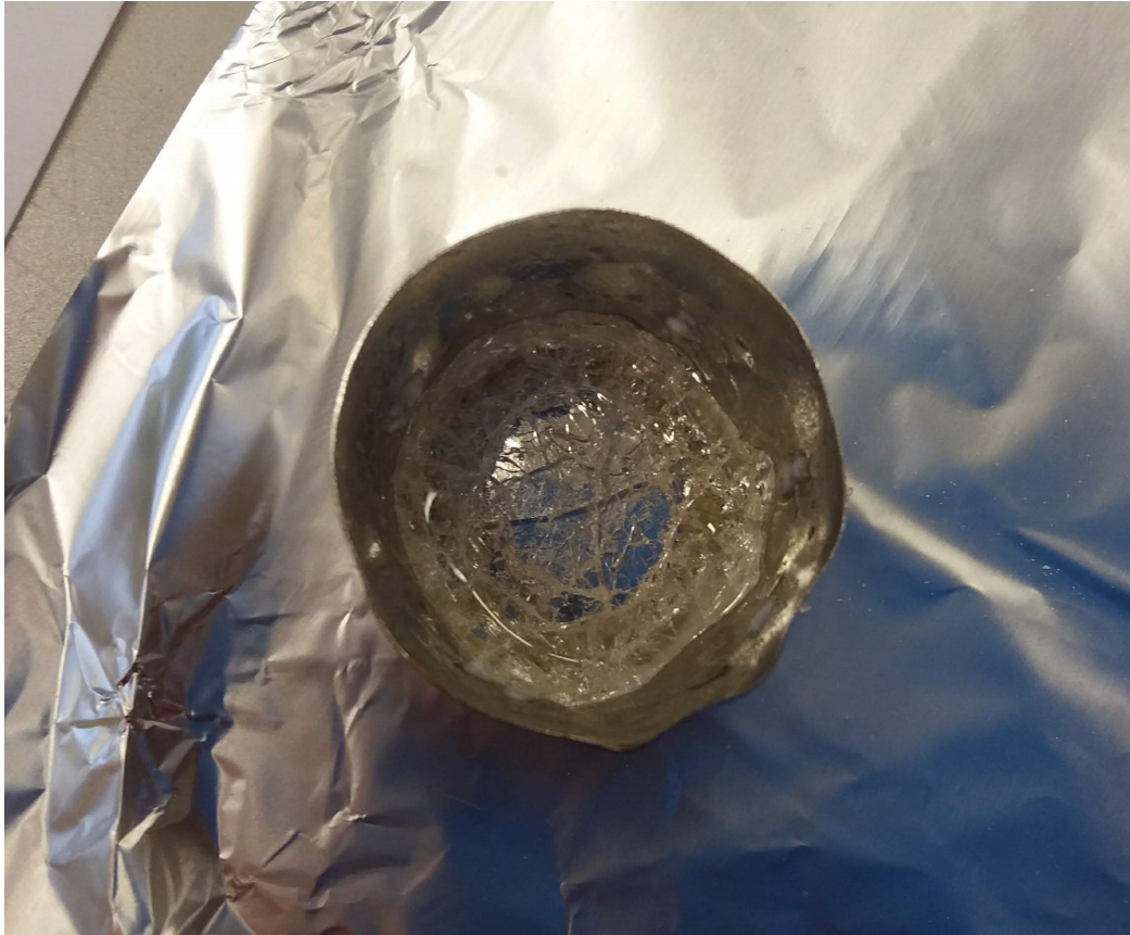
Figure 6-2: Natural diopside glass in a Pt-10%Rh crucible after quenching. The sample looks completely clear and glassy.
