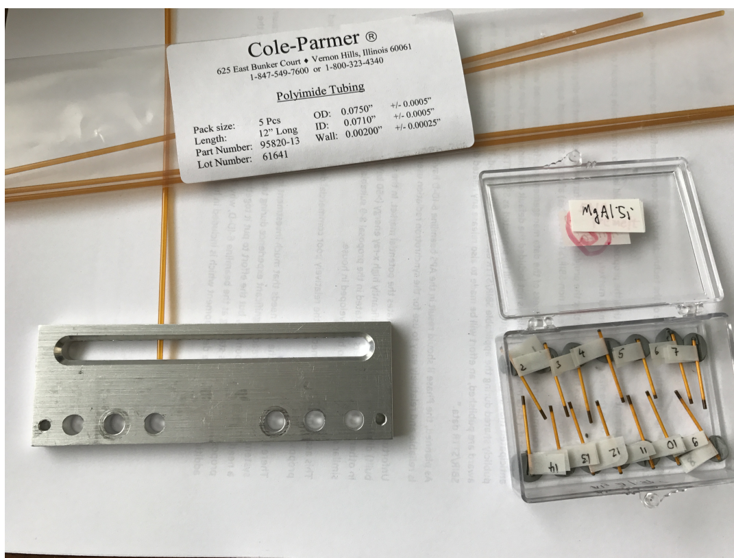
Figure 5-3: MAS samples held in kapton polyimide tubes.
