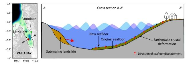
Figure 7. Sketch showing the final dual (earthquake and submarine landslide) model proposed in this
