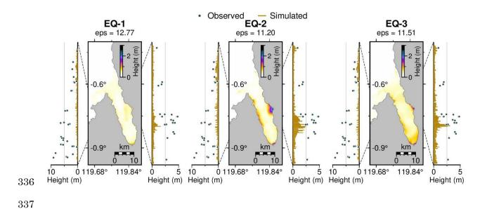
Figure 5. Comparison of simulated and observed runup for three earthquake-only source models EQ1, EQ-2, and EQ-3. The observed data (i.e., circles) is based on Omira et al. (2019). "eps" indicates
