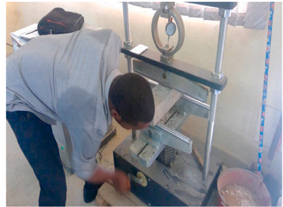
Fig. 2. Flexural test on beams.
