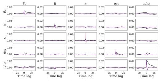
FIGURE 8. Comparison of cross-covariance of training data and generated data with cross-covariance (solid lines on top of each other, numerical error of order  $10^{-16}$ ), covariance or sampled covariance (dashed lines) post-processing and uncorrelated model (dotted line) for test case (ii).
