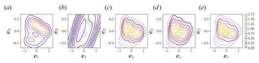
FIGURE 14. Kernel density estimation of the 2-D kernel PCA embedding of the (a) training data and generated data via (b) uncorrelated model, (c) empirical covariance, (d) cross-covariance and (e) sampled covariance post-processing for test case (iii). The embedded training data are shown in grey in all plots. The colour scale representing the density is the same in all plots.
