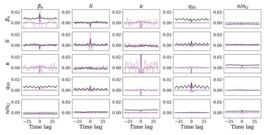
FIGURE 12. Comparison of cross-covariance of training data and generated data with cross-covariance (solid lines on top of each other, numerical error of order  $10^{-16}$ ), covariance or sampled covariance (dashed lines) post-processing and uncorrelated model (dotted line) for test case (iii).
