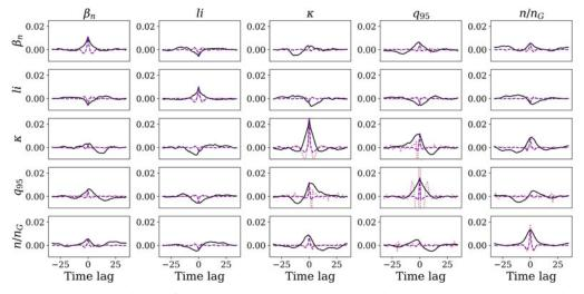
FIGURE 4. Comparison of the cross-covariance in the training and generated data with cross-covariance (solid lines on top of each other, numerical error of order  $10^{-16}$ ), covariance or sampled covariance post-processing (dashed lines) and uncorrelated model (dotted line) for test case (i).
