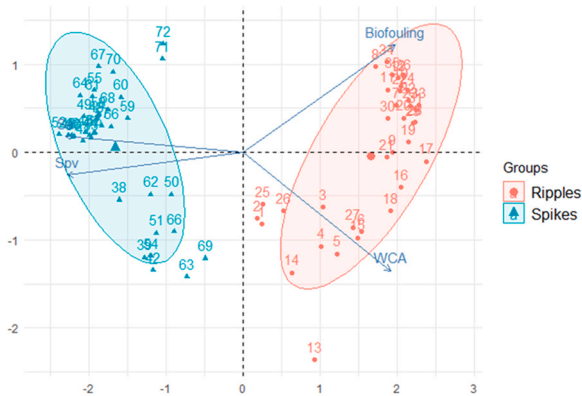
Fig. 6 – PCA biplot visualising relationships between the surface roughness measures ( S_a , S_q and S_{pv} values), WCA and biofouling percentage for each of the surfaces and cleaning conditions. The 95% ellipsoids represent clusters based on surface texture type as the key variable with the following colours for each: spiked (blue) and rippled (red).
