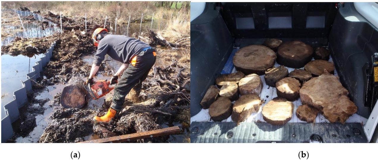
Figure 4. Recovering subfossil bog-pine trees from Wem Moss, Shropshire in March 2015. (a) Sampling tree discs using a chainsaw from well-preserved stumps close to the tree root crowns. Note corrugated plastic barrier inserted into the peat as a hydrological barrier. (b) Seventeen pine disc samples prior to transportation to the Dendrochronology laboratory at Manchester Metropolitan University.
