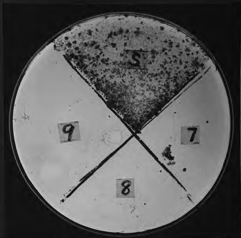
Fig. 7. The effect of Ultra-violet light on T. discoides (arthrospores suspension) Numerals indicate exposure time in minutes. 'S' indicates unexposed sector.
