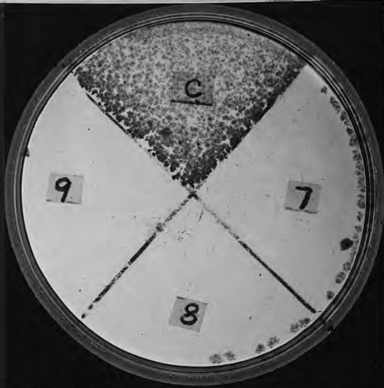
Fig. 7. The effect of Ultra-violet light on T. discoides (arthrospores suspension) Numerals indicate exposure time in minutes. 'S' indicates unexposed sector.
