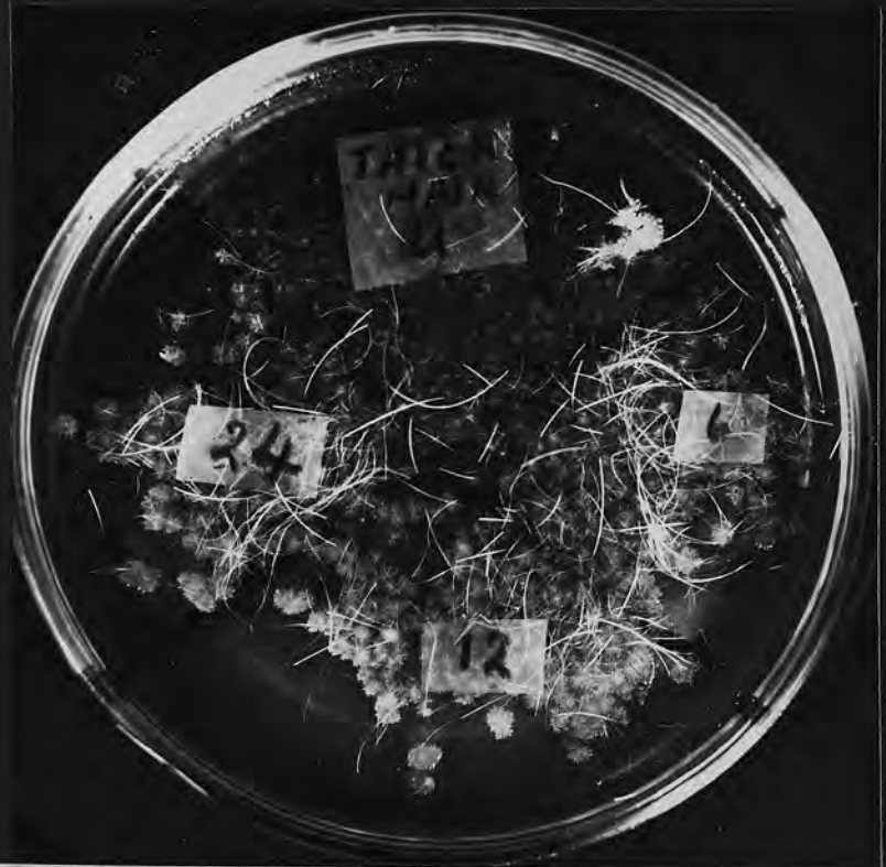
Fig. 15. Protective action of hair on T. discoides exposed to Ultra-violet light. Numerals indicate time of exposure in minutes. 'U' indicates unexposed sector.
