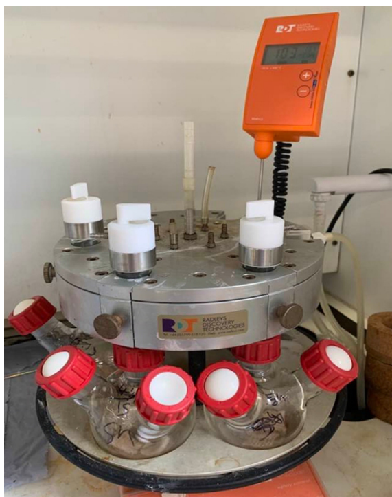
Photo 1. Esterification reaction under water-cooled reflux in Radley Carousel reactor.
