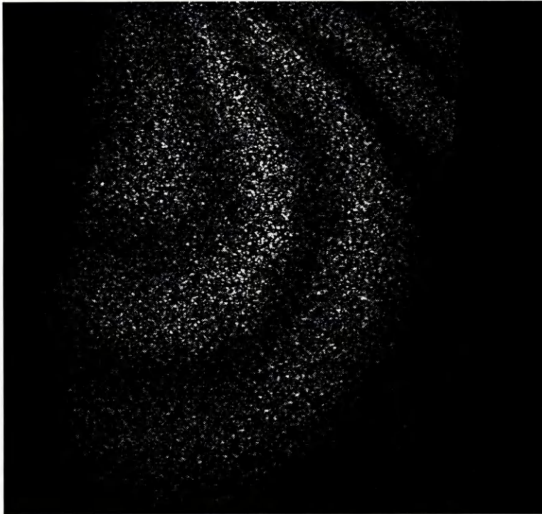
Fig. 6.10 Stroboscopic fringes of turbine blade vibrating at 2 kHz, measured using shearography with 0^\circ phase shift
