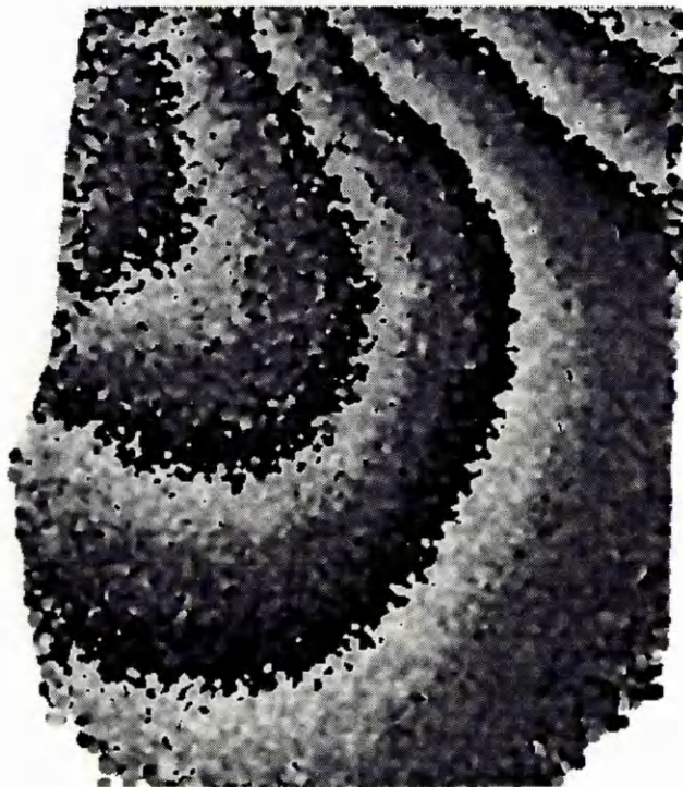
Fig. 6.11 Wrapped phase map calculated from the phase stepped fringes (2 kHz mode)
