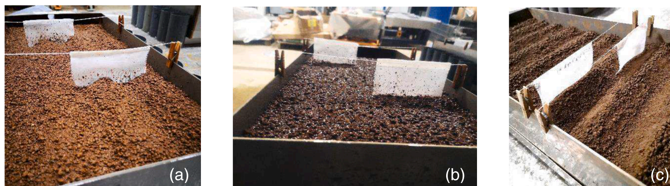
Fig. 3. Capturing soil particles detached by rainsplash on the erosion trays. (a) Collector voiles cut to fit the shape of Treatment A. (b) Two collector voiles placed at the top and bottom of the erosion tray. (c) Two collector voiles put on the ridge and in the furrow of Treatment B.
