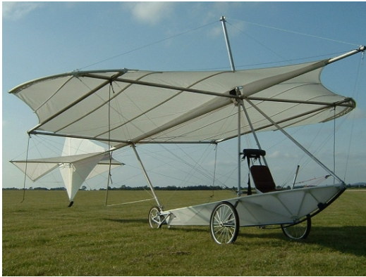
Figure 2.1: The conventional aircraft configuration conceived by G.Cayley, featuring a lifting surface and conventional empennage.
