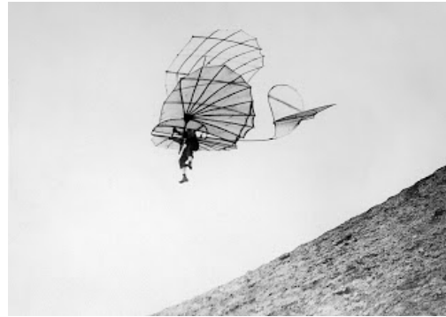
Figure 2.2: O. Lilienthal performed an extensive series of experiments with various glider designs. The results were monitored in a scientific manner and were later used by the Wright brothers.
