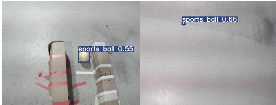
(c) Ball in between two "rail vehicles" (lighter condition). (d) False positive detection (lighter condition).
