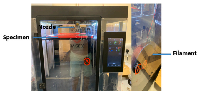
Fig. 3. 3D printing by Raise 3D Pro2.
