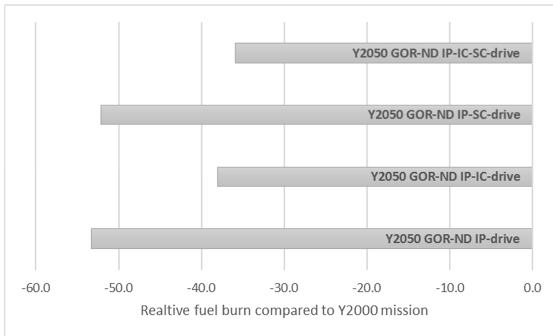
Figure 5- 70: Overview of the relative fuel burn of all Y2050 GOR-ND IP configurations relative to a year 2000 short range mission
