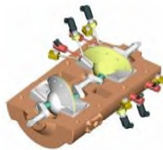
Figure 2- 5 : proposed arrangement of a dual disc nutating disc engine system [79]
