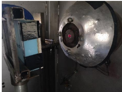
Fig. 5. Multi-layer target setup in ELVIS before being impacted by 5 mm steel projectile at 400 m/s. The target face is Aluminium, followed by Kevlar-Epoxy, Polyurethane foam, and polycarbonate.
