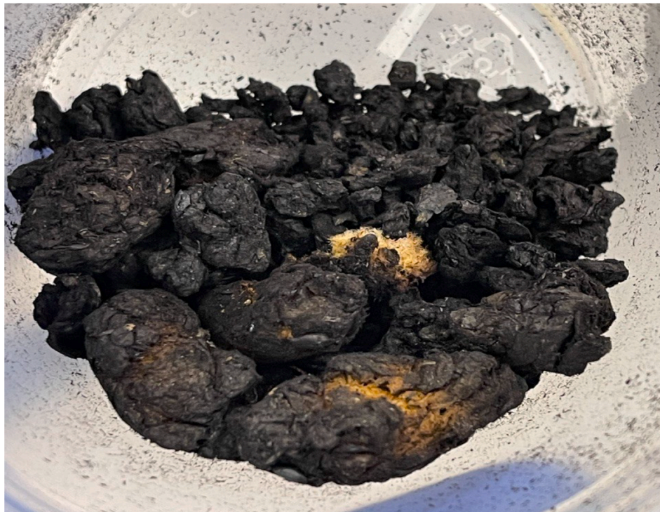
Fig. 7. Incomplete conversion of char obtained from test 1 at 375 °C.
