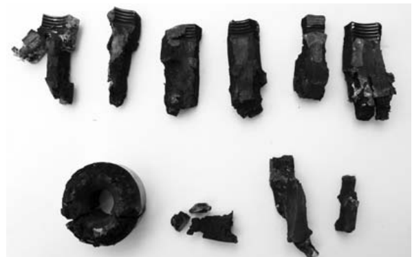
Fig. 7. Fragments of the vehicle in the detonative test.
