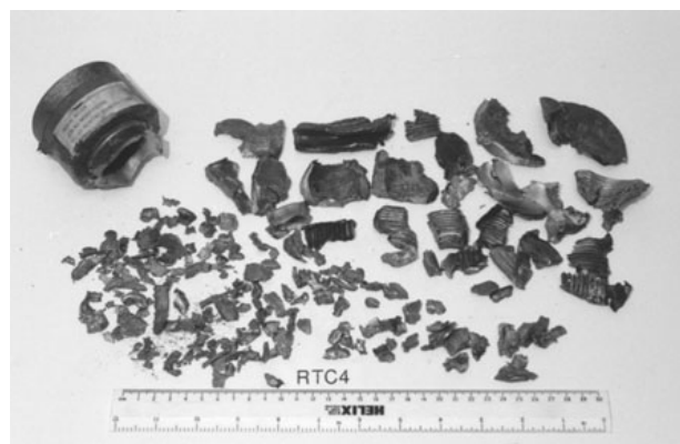
FIGURE 8. Vehicle remains from partially-heated RDX/TNT experiment.
