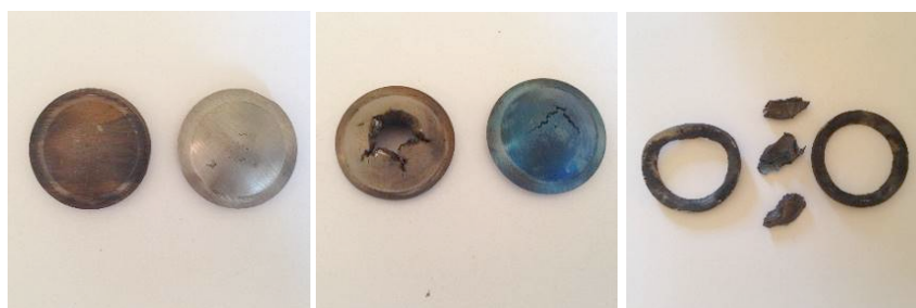
FIGURE 3. Photographs of steel end plates recovered from separate tests showing increased violence from left to right.
