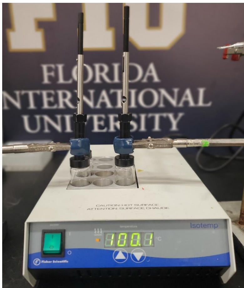
Figure 75. TPPO extraction setup using a heating block.
