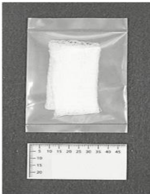
Figure 26. Image of a COMPS device containing a gauze pad inside of a sealed low-density polyethylene (LDPE) polymer bag. Target compounds are spiked onto the gauze pads prior to sealing [125]
