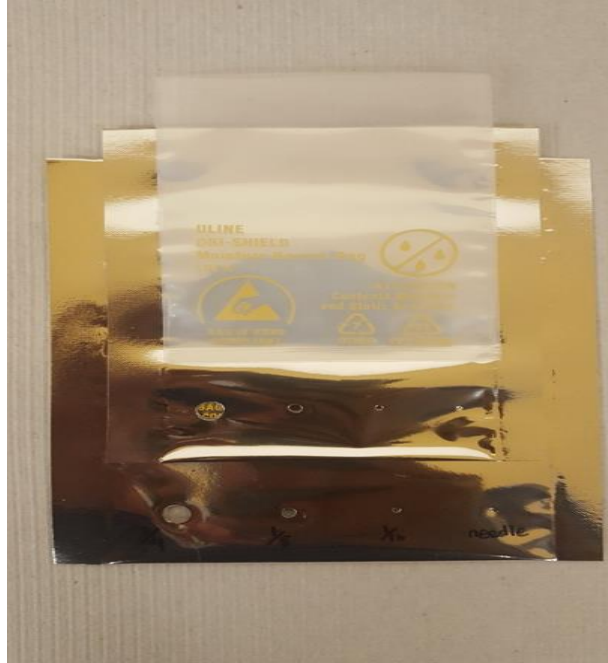
Figure 81. Low density polyethylene (LDPE) bag (top) alongside a perforated Aluminum bag.
