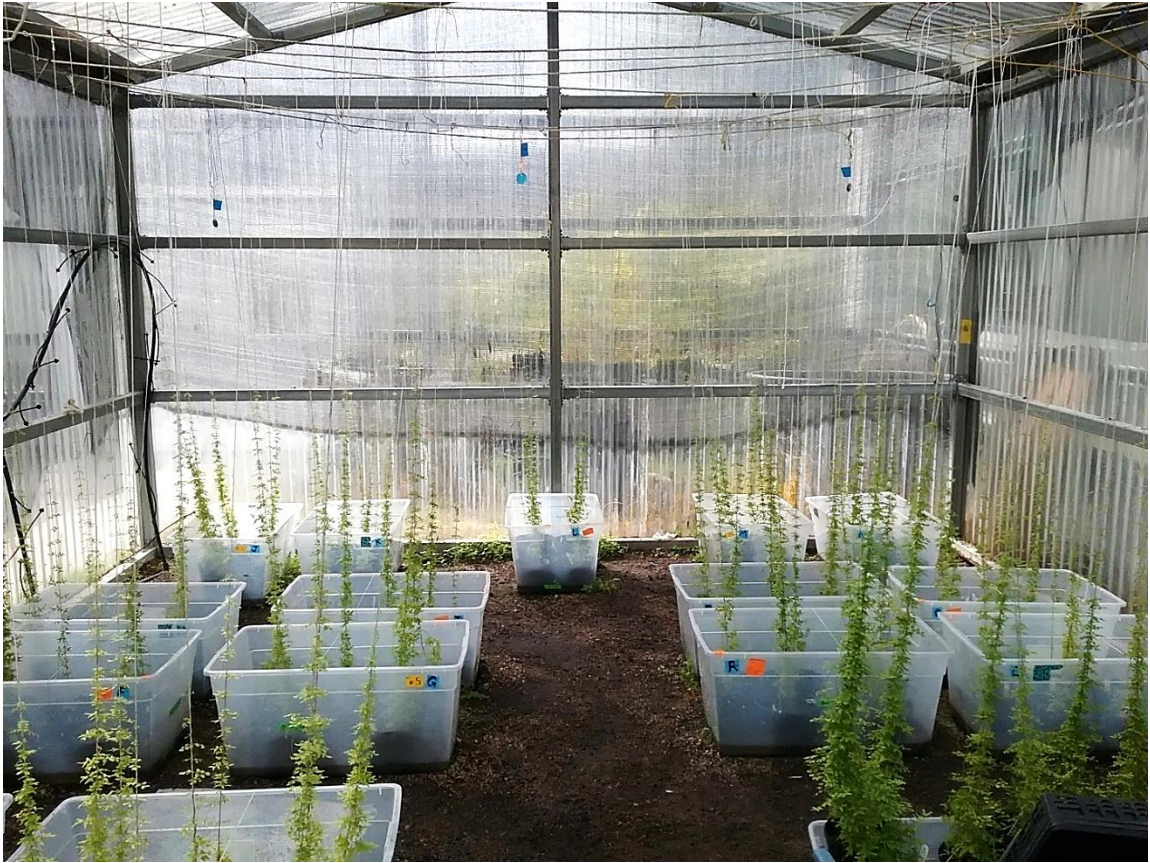
Figure 3.1. Experimental set-up for L. microphyllum salinity experiment. Eighteen bins (not all pictured), each with 5 potted plants sitting in either 0, 5, or 10 ppt solution. Polypropylene twine suspended from a rope lattice supports each plant's twining growth. Several thermochrons suspended from the rope lattice recorded hourly temperature.
