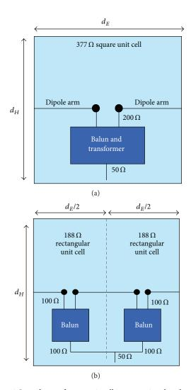
FIGURE 6: Impedance of array unit cell is proportional to the aspect ratio of  $d_E/d_H$ . Splitting the cell vertically into two halves, the impedance is reduced by a factor of two. Combining the halves in parallel reduces the impedance by another factor of two (power divider from  $50~\Omega$  to  $100~\Omega$ ). (a) Square  $377~\Omega$  unit cell and (b) two  $188~\Omega$  "half" unit cells from [48].
