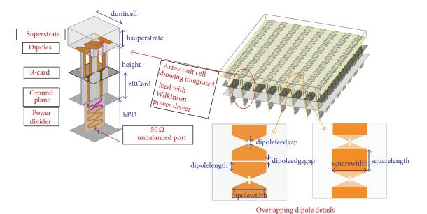
FIGURE 5: Illustration of the tightly coupled dipole array (TCDA) integrated with a balun to create the TCDA-IB array. Enhanced coupling between dipole is achieved using overlapping dipoles at the array's surface. The Marchand-type balun is depicted to the left and a single feed is used to feed a pair of dipoles (creating the unit cell) to double the impedance from the Wilkinson divider for improved matching at the dipole terminals.
