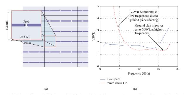
FIGURE 4: VSWR for a tightly coupled dipole array (TCDA) when radiating in free space or in presence of a metallic ground plane from [46].
