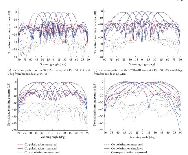
(c) Radiation pattern of the TCDA-IB array at  $\pm 45$ ,  $\pm 30$ ,  $\pm 15$ , and 0 deg from broadside at 1.2 GHz
