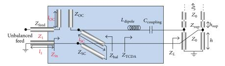
Figure 19: Simplified Marchand balun equivalent circuit (see [48]).
