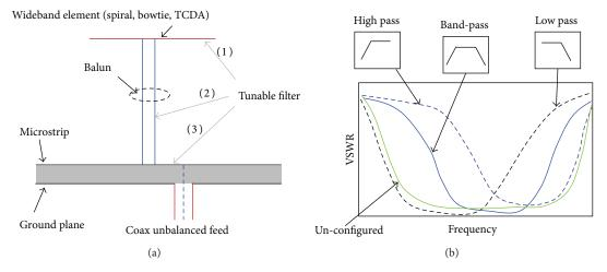
FIGURE 16: Bandwidth reconfiguration concepts: (a) tunable filtering integrated in the aperture (1), feed (balun) (2), or the ground plane (3); (b) representative bandwidth response due to reconfiguration.
