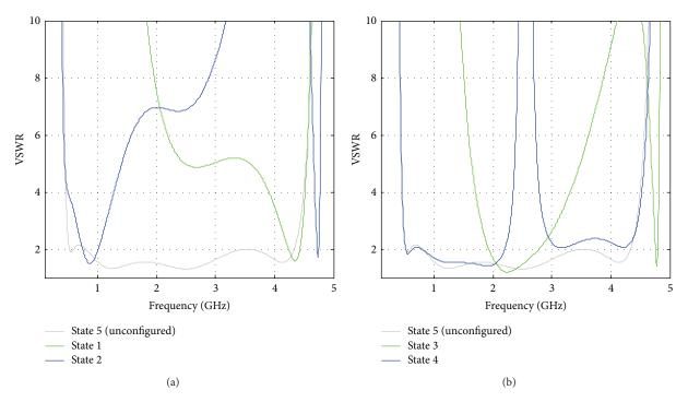
FIGURE 21: VSWR versus frequency for Table 2 reconfiguration states.
