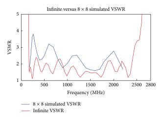
FIGURE 12: VSWR comparison of the infinite versus  $8 \times 8$  finite TCDA-IB array defined in Figures 5–9. It is noted that the truncation effects of the edge elements of the  $8 \times 8$  array are responsible for the higher VSWR associated with the  $8 \times 8$  array.
