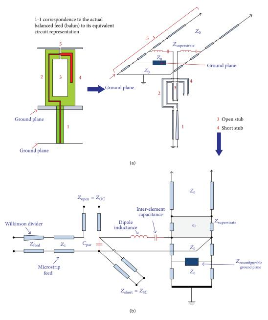
FIGURE 17: Equivalent circuit representation of the TCDA-IB array in Figure 5. The top graphic provides a one to one correspondence between the Marchand balun in Figure 2 and its equivalent transmission line circuit representation. The bottom circuit is a recasting of the equivalent transmission line circuit into a more typical RF circuit showing the open  $(Z_{\rm OC})$  and short circuit  $(Z_{\rm SC})$  impedances of the balun itself.
