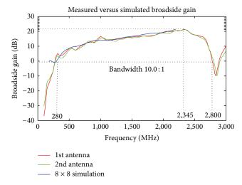
FIGURE 11: Measured and simulated realized gain at broadside (copol/E-pol data) for the TCDA-IB array whose geometry is presented in Figures 5–10. The agreement among all 3 gain curves provides substantial confidence in the validity of the measured performance. Small fluctuations in the realized gain are attributed to the horn used for calibration during measurements.
