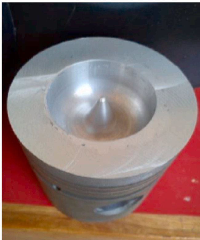
Fig. 6. Toroidal combustion chamber [13] (Adapted with permission from the publisher).
