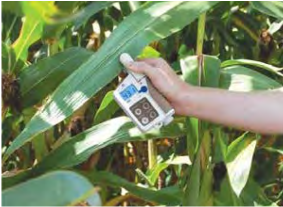
Figure 21.3. In-field sensors used to measure nitrogen status of leaves and canopies. Left: leaf chlorophyll (SPAD) sensor. Photo by Konica Minolta. Right: proximal canopy sensors. Photo by Trimble Agriculture.
