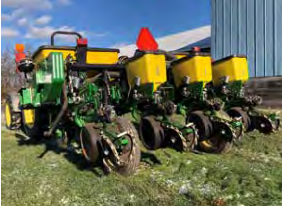
Figure 16.7. A modern row-crop planter for conservation tillage systems. Coulters in front and closing wheels in the back allow for seed placement without soil preparation; equipment positioning is controlled by a GPS system; seed depth is controlled by hydraulics; seed is delivered by vacuum; and seed placement is digitally monitored. Photo by Larissa Smith.
