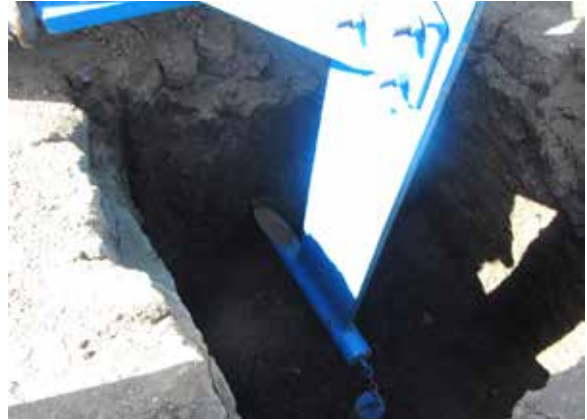
Figure 17.18. A mole drain in a clay soil (left) is created with the use of a mole plow with a “bullet” and expander on a chain (right).
