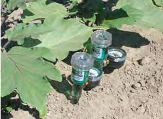
Figure 17.11. Tensiometers used for soil moisture sensing in irrigation management. Photo courtesy of the Irrrometer Company.
