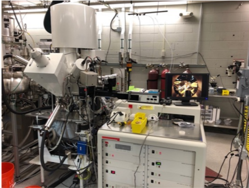
Figure 8: Kratos Ultra DLD surface analysis system in ANSLab used for XPS measurements
