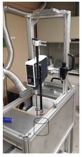
Figure 5.1. The stirrer mounted on an aluminum frame above the aluminum enclosure that contains the induction furnace. The black cylinder indicates the position of the crucible in the enclosure box.
