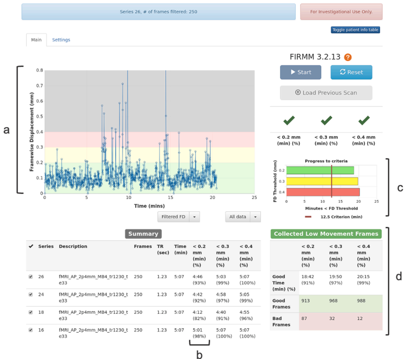
Fig. 1. FIRMM prototype software available in 2017 and used for data collection in Cohorts 4 and 5. (a) Motion Trace: plot of FD values for each frame. (b) Minutes and percentage of fMRI data below 0.2 mm for a given scan run; (c) Progress to criteria: total minutes of data collected compared to a predetermined minimum goal; and (d) Collected Low Movement Frames: running total of minutes, percent, and number of frames of data below the set threshold.
