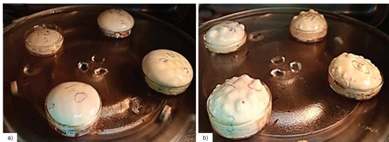
Figure 2. The samples during foaming and curing via MH: (a) at 12 minutes at 600 W and (b) at 15 minutes at 600 W.
