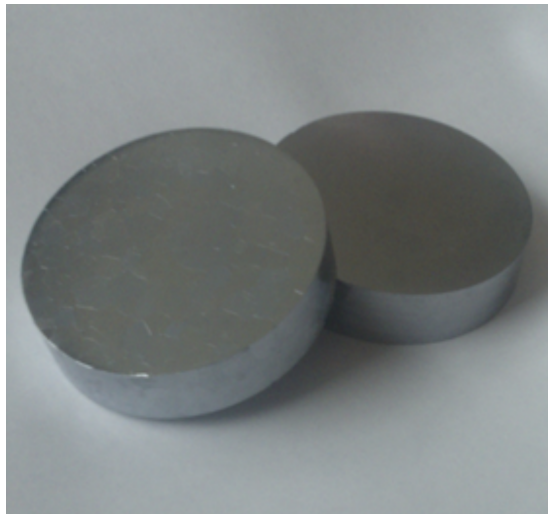
FIG. 2: Two vanadium discs after multifold electron beam melting (EBM).
