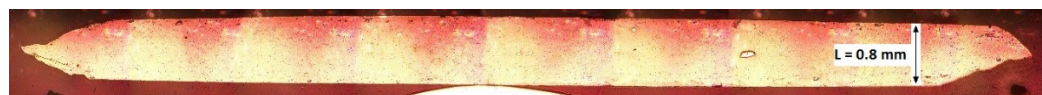
Figure 3. Optical micrograph taken on the cross-section of the HPT disk obtained after N = 5 rotations.
