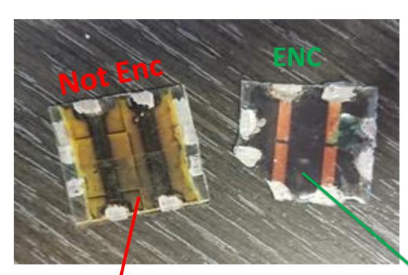
Yellowing of the Encapsulated device perovskyte layer preserved their brownish after a couple of days due to  $O_2$  and  $H_2O$
