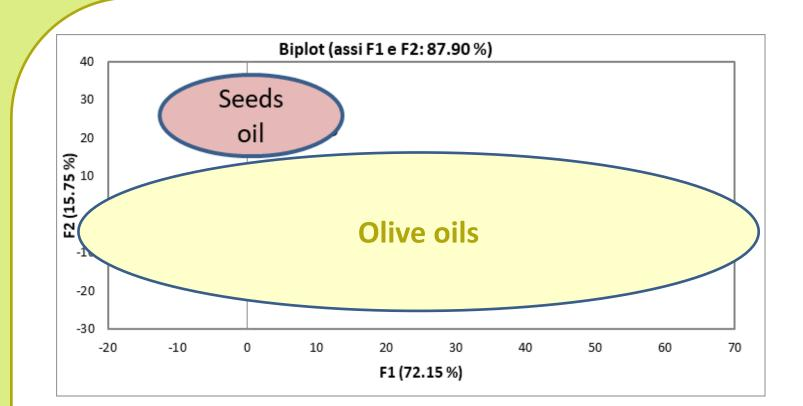
The features observed in the voltammograms reflect the reactions of electroactive compounds (such as polyphenols), which are present in the oils mixed with the carbon matrix. For this reason, the voltammetric responses of the electrodes are specific for each type of oil.
