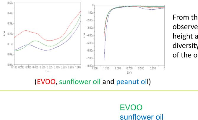
From the comparison of the profiles obtained, it is possible to observe differences in the number of peaks present, in their height and in the potential to be observed, which highlighted the diversity in the content and nature of the antioxidant compounds of the oils with different plant origins.
