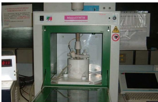
Figure 2. Simultaneous US/MW irradiation (horn made of PEEK ® ).
