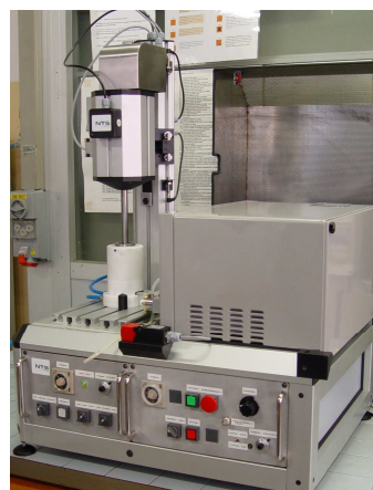
Figure 3. Loop reactor for sequential US/MW irradiation.
