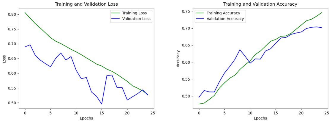
Figure 6.1: Loss and Accuracy plots related with the training and validating processes with the Flow Gated Network , trained from scratch on the YNF dataset. These results were achieved through a process of 25 epochs, 0.0001 for learning rate, no data augmentation, with the optimizer SGD, batch size of 2, the frame rate of four, and weight decay on the last two dense layers.
