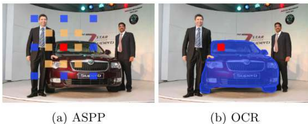
Figure 2.11: Visual representation of multi-scale context (with ASPP) and OCR context. The context is for the pixel marked as red. (a) ASPP: The context is a set of sparsely sampled pixels marked with yellow and blue. The pixels with different colors correspond to different dilation rates. (b) OCR: The context is expected to be a set of pixels lying in the object (marked with color blue) [57].
