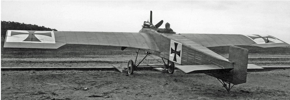
Figure 3.6: Junkers J1 with its all-metal airframe [7]
