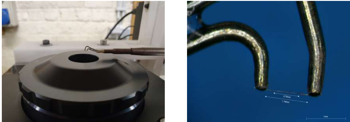
Figure 4.3: Probe mounted on the external calibrator (left) and wire detail (right)
