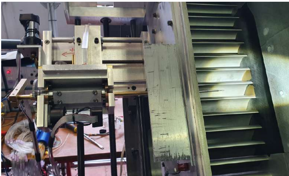
Figure 3.3: Hot-wire placed in traverse the support system
