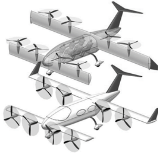
Figure 1.1: Representation of a passenger Vectored Thrust Vtol concept in hover (top) and flight (bottom) from [3]
