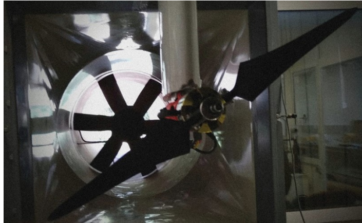
Figure 3.19: Propeller s9000 14 positioned to be tested in UBI subsonic wind tunnel
