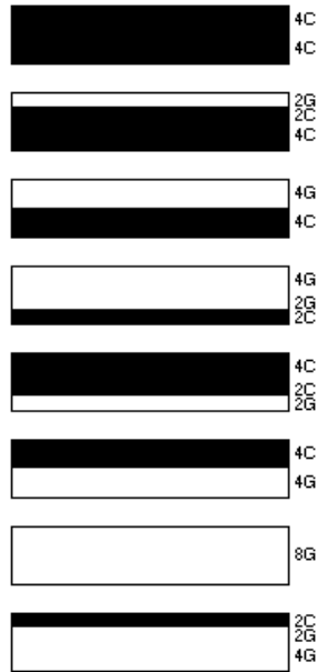
Figure 5.8: Illustration of the decrease in strength in function of the evolution of the glass and carbon fibre layers in the laminate
