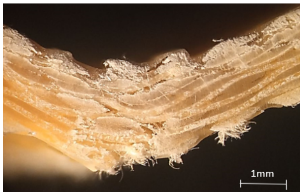
Figure 5.6: Failure mode of a kevlar fibre reinforced laminate (8K)
