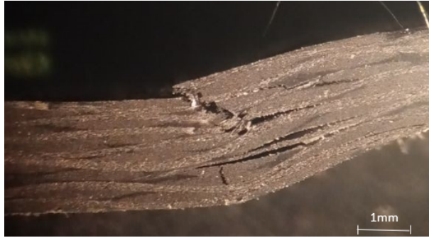
Figure 5.4: Failure mode of a carbon fibre reinforced laminate (8C)
