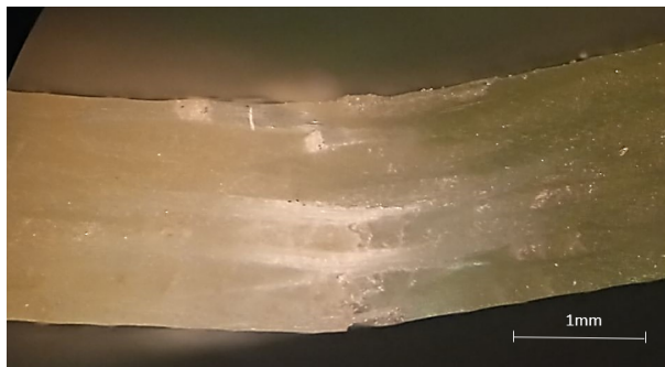
Figure 5.5: Failure mode of a glass fibre reinforced laminate (8G)
