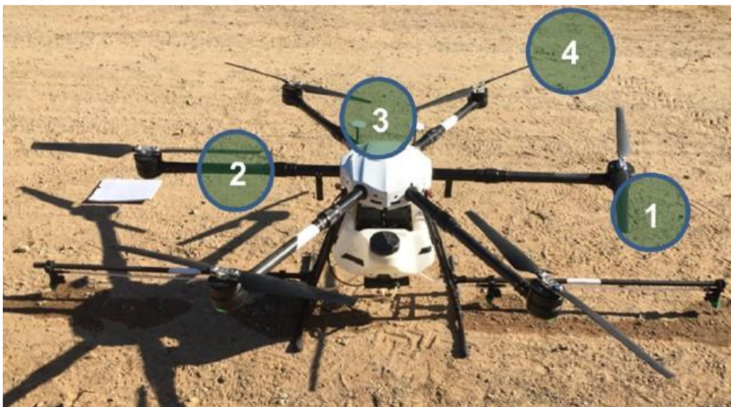
Figure 23 – Locations of the pesticide depositions found on the UAV: (1) spray boom, (2) arms, (3) central hub, (4) rotor blades – Source: [37]
