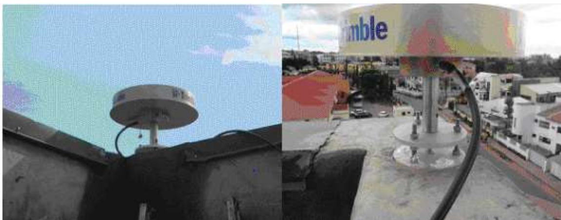
Figure 2. 4: GNSS Stations Located on OSGoF and UNILAG Buildings Source: Fernandes et al., (2010)
