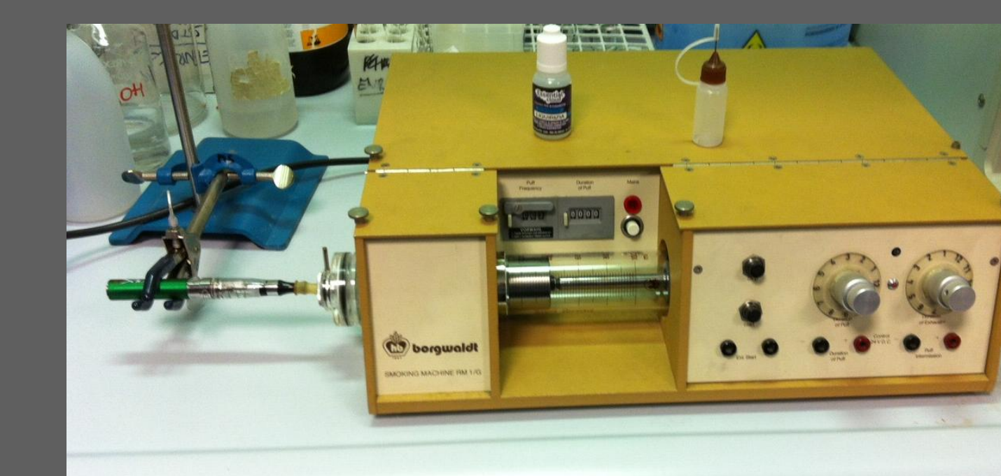
Figure 4: Smoking machine generating aerosol from e-cigarette
