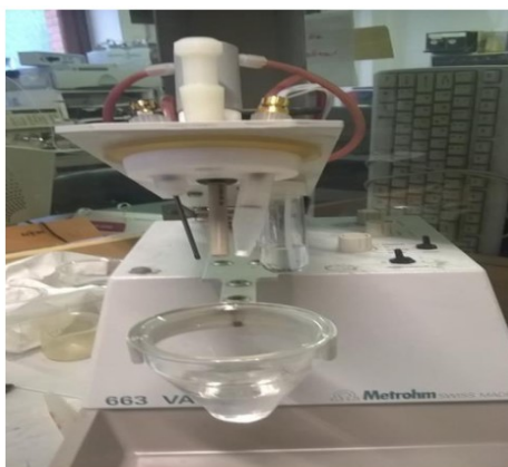
Figura 1. Electrolytic cell in a conventional voltammetric analyzer.
