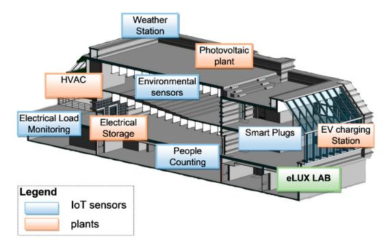
Figure 4. eLUX lab and the IoT assets.
