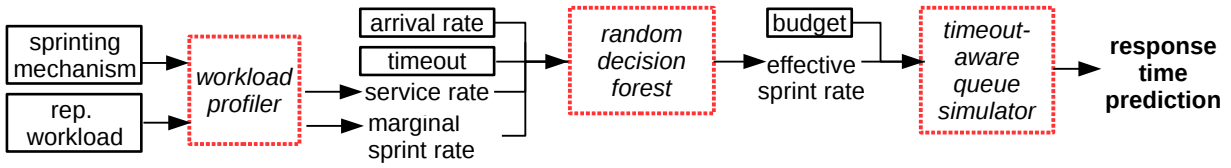
Fig. 2: Our approach combines workload profiling, queue simulation and machine learning (shown in red dotted squares). Black squares show inputs provided by users.
