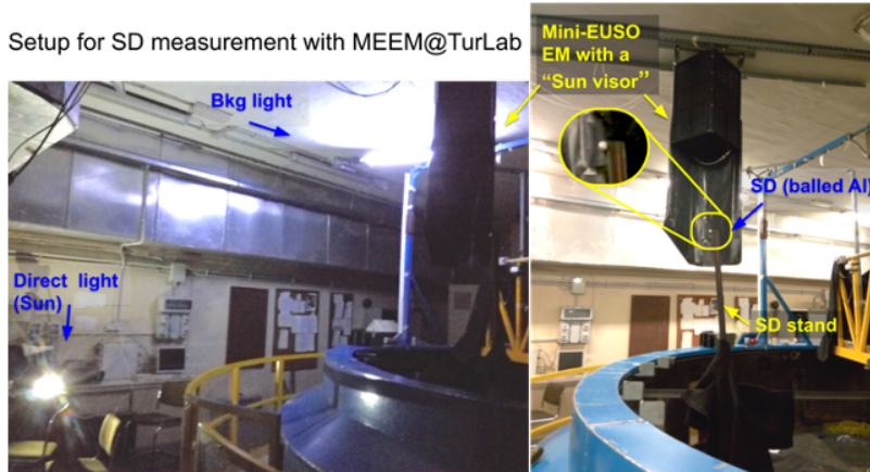
Fig. 21 TurLab setup for SD detection by the Mini-EUSO EM. The FS of Mini-EUSO EM apparatus is protected by a “Sun visor” to avoid the direct light from the white LED which is fixed outside of the tank, mimicking the Sun light. An aluminum ball under the apparatus of Mini-EUSO EM is attached to a solid stand which is fixed to the bottom of the tank. As the tank rotates, the aluminum ball moves within the EUSO@TurLab apparatus FoV being illuminated by the LED. Image adapted from [33].
